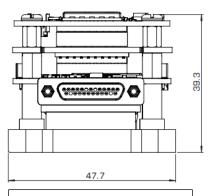
Device side: 25-pin connector MDSM-25PE-Z10-VR17
